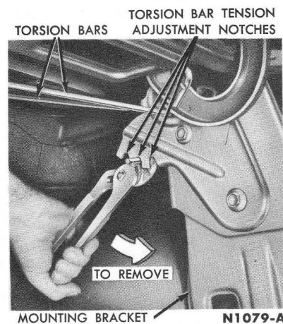
FIG. 15—Deck Lid Torsion Bar Replacement
