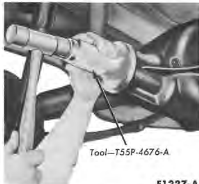
FIG. 16—Drive Pinion Flange Seal Installation
