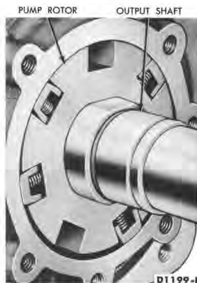
FIG. 26—Rear Pump Rotor Alignment
