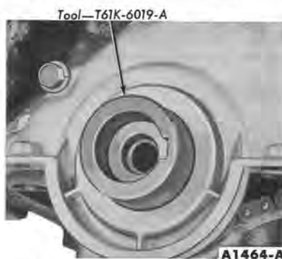
FIG. 53—Cylinder Front Cover Alignment
