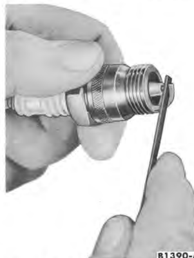
FIG. 17—Cleaning Plug Electrode
