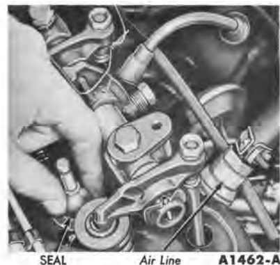
FIG. 50—Valve Stem Seal Removal
