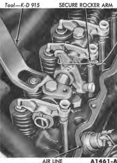
FIG. 49—Compressing Valve Spring
